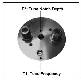
Tuners for VR7-FM-2501 series —Adjusts Frequency (T1) and Depth (T2) of notch
